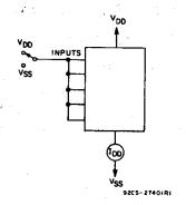
Fig. 12 - Quiescent-device-current test circuit.
