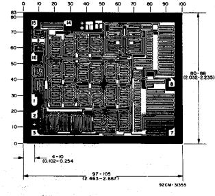
Chip dimensions and pad layout for CD4045B
