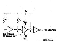
Fig. 11 - Typical RC circuit.
