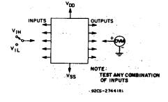
Fig. 13 - Noise-immunity test circuit.
